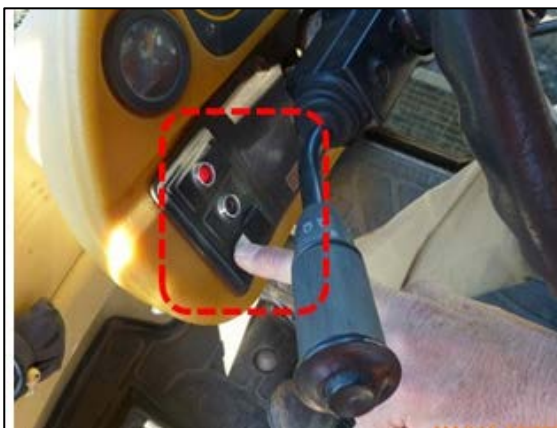
Figure 3. One horizontally-oriented (left / right) rocker switch (finger shown pressing to left side); 2 status lamps; no labels.
