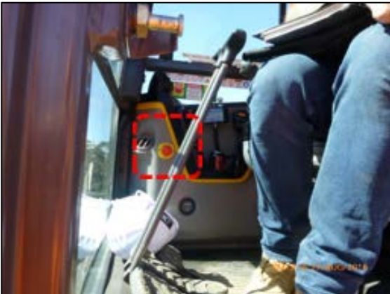
Figure 13. Interior Emergency Stop push-button: located low on the right cab interior wall; well outside driver's primary visual field.
