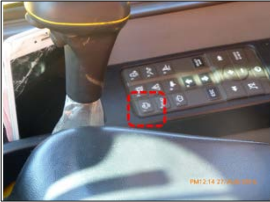
Figure 11. Copy of Figure 2 showing close proximity of numerous soft-key press-buttons for differing functions. See Figure 12 (at right) for close-up.
