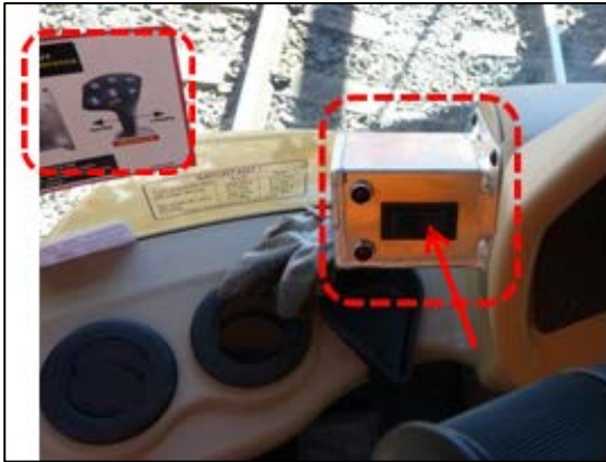
Figure 5. One horizontally-oriented (left / right) rocker switch (arrowed); 2 status indicator lamps; no labels. A separate windscreen sticker (at the left of photo) with somewhat convoluted instructions for use (see photo at right). Located on the left side of the front console.
