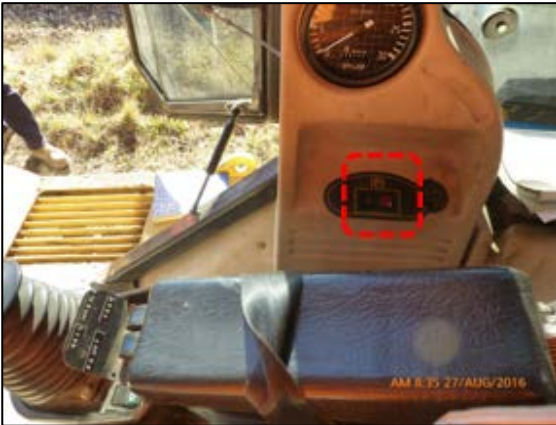
Figure 17. Most vehicle park brakes were located low and to the right rear side of the driving position, well outside of the driver's visual field.
