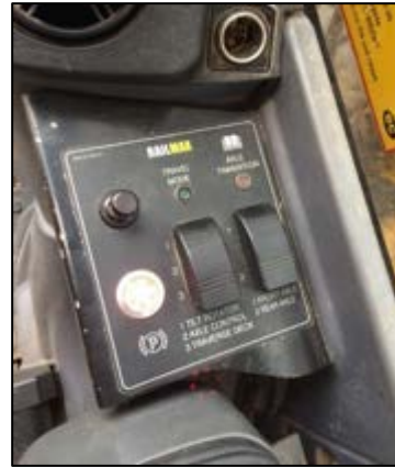
Figure 18. Park brake for RGS co-located with the RGS operation switches.
