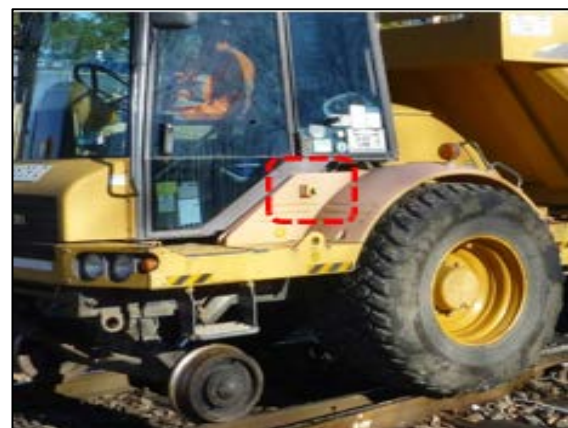
Figure 16. Exterior Emergency Stop push-button: located on the left side of the vehicle; requires reaching in close proximity to rear road wheel in order to activate.
