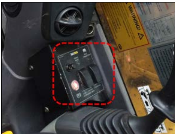
Figure 5. One horizontally-oriented (left / right) rocker switch (arrowed); 2 status indicator lamps; no labels. A separate windscreen sticker (at the left of photo) with somewhat convoluted instructions for use (see photo at right). Located on the left side of the front console.
