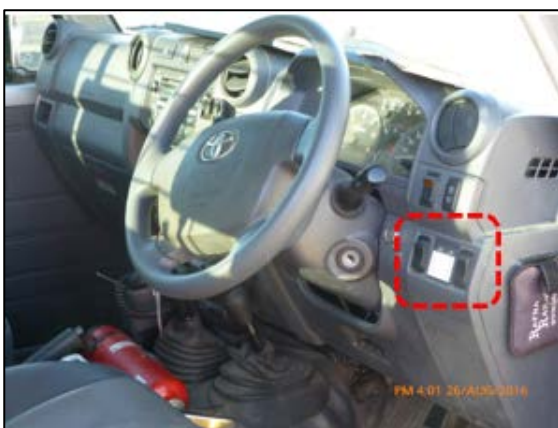
Figure 9. Older type RRV: 2 vertically-oriented rocker switches; 2 status indicator lamps; dedicated labelling.
