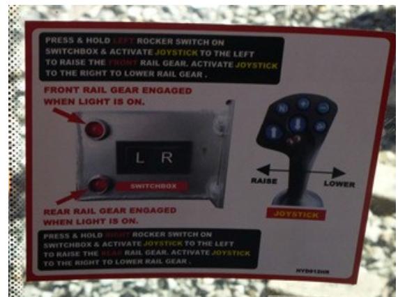
Figure 6. The separately located instructions sticker (refer RGS in photo at left). The left / right rocker switch (which activates front and rear rail wheels, respectively) is labelled on the sticker as “left / right” rather than “front / rear”.
