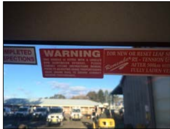
Figure 34. Warning and information stickers placed on interior of vehicle's windscreen.
