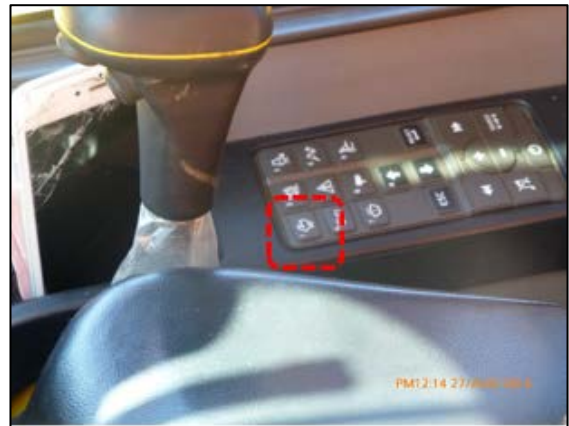
Figure 2. One press button; no status indications; one un-labelled and ambiguous symbol on button.
