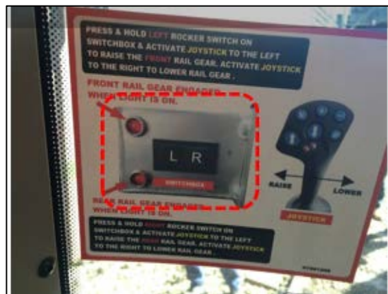
Figure 36. An instruction sticker in the same RRV showing the actual RGS controls. These are completely different to those shown in the Operating Manual held in the vehicle.
