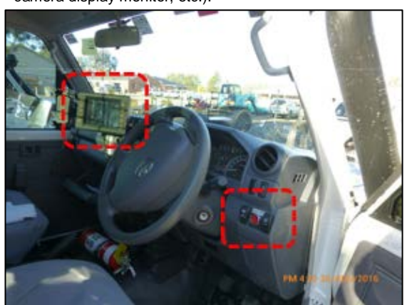
Figure 10. Newer type RRV: Touch-screen interface with RGS controls (at left); separate “Hyrail” park brake release button (at right).
