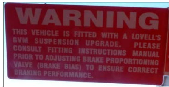
Figure 38. Close up of the “brake proportioning valve” warning sticker.
