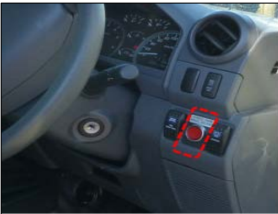
Figure 19. Hi-rail parking brake release button ( not application button) located low and to the right of the steering wheel on the front dash housing. Park brake application was activated via the touch screen.
