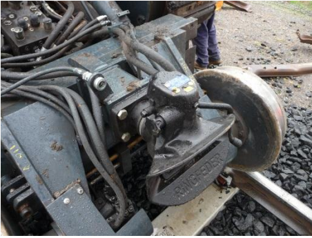
Figure 2: Ringfeder type coupler
