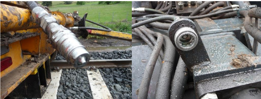
Figure 3 and 4: Hydraulic coupling
