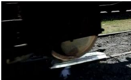
Wheel on derailer
