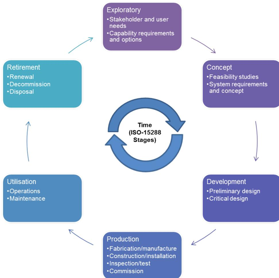
**Figure 2: Asset life-cycle phases of ISO/IEC 15288-2008**
